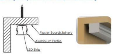
CRecessed Mounting by drilling hole through the extrusion and fixing directly onto the pre-made channel
