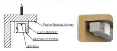
BMounting by drilling hole through the extrusion and fixing directly onto the wall - most professional looking
